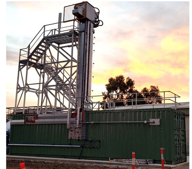
Direct electrical heating has been proven at pilot scale at the Calix Technology Centre.
