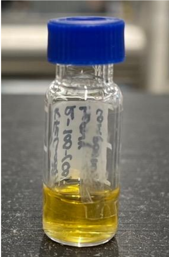
Syn-diesel from syn-crude used to prepare surfactant pre-cursors
